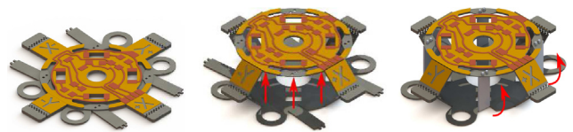
Fig. 5. PCMEMS multisensor structural assembly: (left) post-fabrication after release cuts are made, (middle) axisymmetric Sarrus linkages guide assembly of sensor along z -axis, (right) interlocking stiffeners are folded into corresponding slots to transmit load to flexural members.
