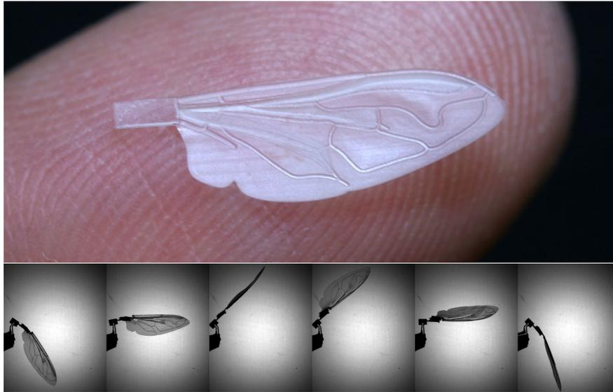
**Fig. 6** Photo of a micromolded polymer wing mimicking the features of a *Eristalis* wing (top). This wing was created in a single molding step and includes veins ranging from  $50\text{-}125\mu\text{m}$  thick,  $100\mu\text{m}$  corrugation, and a  $10\text{-}20\mu\text{m}$  membrane. A sample of the wing motion (dorsal perspective) at  $150\text{Hz}$  flapping frequency taken from a high speed video (bottom).
