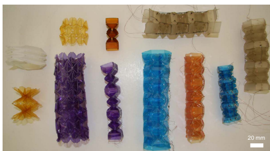
Fig. 6. A collection of origami robots fabricated by the proposed procedure. From left to right, the first column displays axial springs, second column shows the negative Poisson's ratio structures, and the rest are robotic worm bodies in various shapes and sizes. The horizontal robot is built for the origami worm case study.
