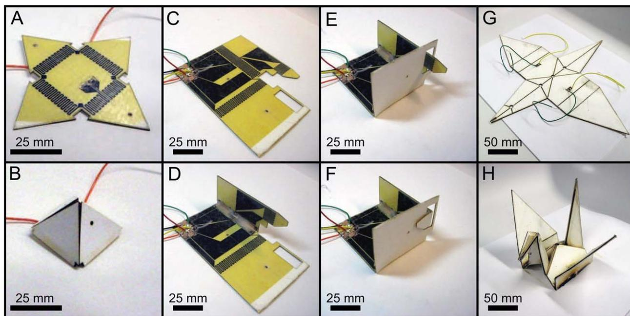
**Fig. 6** (A and B) A pyramid folded through simultaneous activation of four hinges via two amperes supplied to a series of resistive circuits. (C–F) A locking slot and tab assembly. This fold is only possible with sequential folding. (G and H) A crane, created with a combination of sequential and simultaneous folding.
