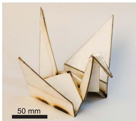
**Fig. 1** An origami-inspired self-folding crane. This structure began as a two-dimensional composite of paper, prestretched polystyrene, and a copper circuit etched onto polyimide. Joule heating resulted in self-folding in three minutes.
