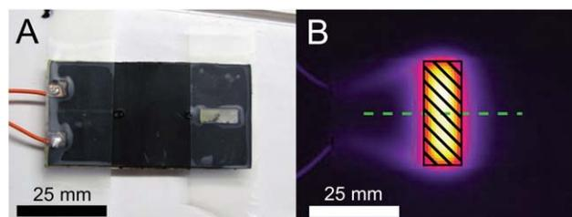
**Fig. 7** The experimental setup used to measure the hinge SMP temperature, viewed in the visual spectrum (A), as well as through a thermal camera (B). The core temperature was determined by averaging the temperature of each pixel within the striped box. The marginal temperature was determined by measuring the temperature profile along the dashed line.
