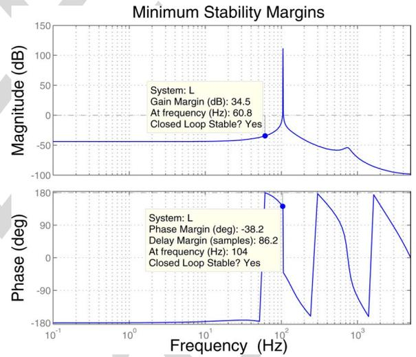
Fig. 13. Estimate  $\hat{L}(z) = -\hat{P}(z)Q(z)$  of the loop-gain function  $L(z) = -P(z)Q(z)$ , computed using the LTI equivalent representation associated with Case 2. The yellow tags indicate the classical minimum stability margins.
