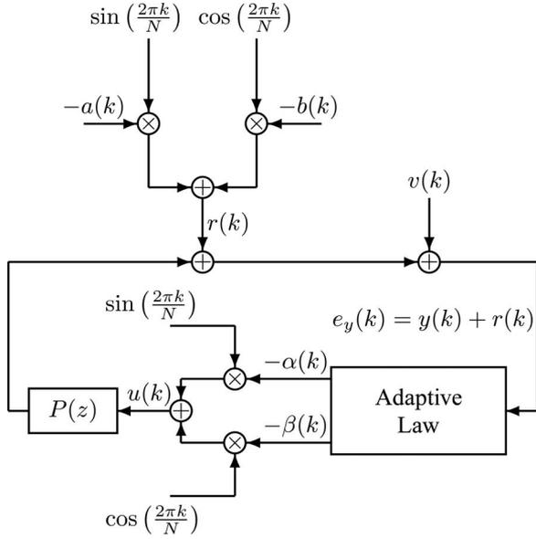
Fig. 5. Adaptive feedforward cancellation (AFC) scheme used for rejecting  $r(k)$  and tracking  $y_d(t)$ .
