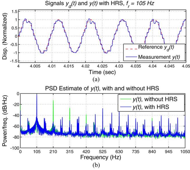
Fig. 9. Case 3. *Upper Plot*: Time series of  $y_d(t) = A_r \sin(2\pi f_r t)$  and  $y(t)$ , using the HRS, with  $A_r = 1$  and  $f_r = 105$  Hz. *Bottom Plot*: Comparison of the estimated PSDs of the measured outputs  $y(t)$ , with and without using the HRS.
