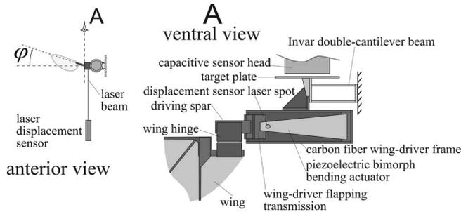
Fig. 2. Diagram of experimental setup for measuring lift forces and actuator displacements. The wing-driver is attached to an Invar double-cantilever beam, whose deflection is measured by a capacitive displacement sensor. This deflection is proportional to the lift force. The actuator displacement is measured using a CCD laser displacement sensor (LK-2001 fabricated by Keyence). For details on the force sensor see [15].
