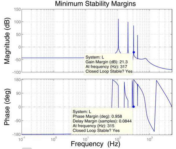
Fig. 15. Estimate  $\hat{L}(z) = -\hat{P}(z)Q(z)$  of the loop-gain function  $L(z) = -P(z)Q(z)$ , computed using the LTI equivalent representation associated with Case 3. The yellow tags indicate the classical minimum stability margins.
