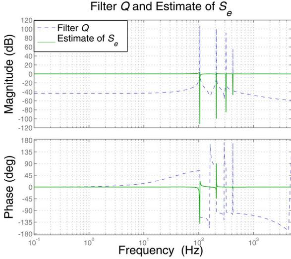
Fig. 14.. Filter  $Q(z)$  and estimate  $\hat{S}_e(z) = [1 - \hat{P}(z)Q(z)]^{-1}$  of the error sensitivity function  $S_e(z)$ , using the LTI equivalent representation associated with Case 3.
