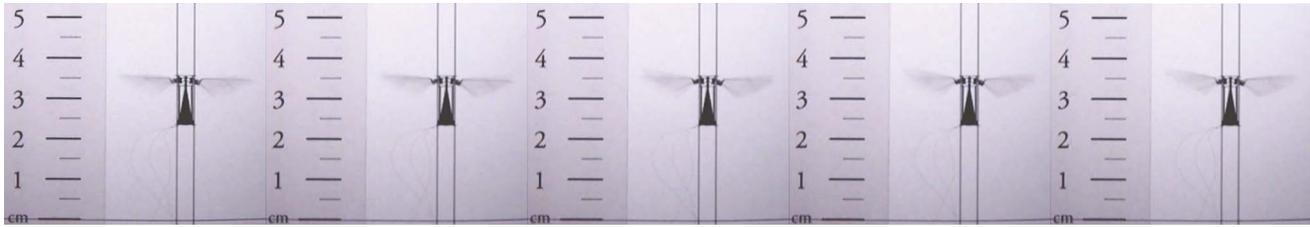
Fig. 25. Sequence of video frames showing a flapping-wing flying microrobot hovering at an altitude of 2.5 cm. The side ruler is placed as a rough reference not for exact measurement of the flying robot's altitude. The exact vertical position  $x(t)$  is measured using a laser displacement sensor. The sampling time at which the frames were taken is approximately 31.9 ms. The complete experiment is shown in the supporting movie S1 at [35].
