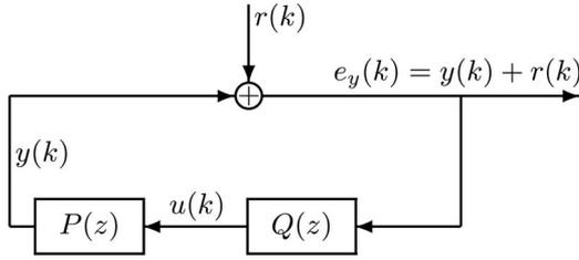
Fig. 11. Equivalent IMP-based LTI model of the AFC scheme in Fig. 5, assuming  $v(k) = 0, \forall k$ .
