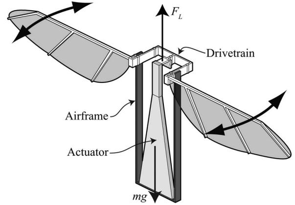
Fig. 1. Illustration of a typical Harvard Microrobotic Fly, similar to the one in [1]. This particular design is described in [14] (drawing courtesy of P. S. Sreetharan).
