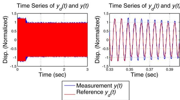
Fig. 23. Comparison of the time series of the experimental  $y_d(t)$  and  $y(t)$ , generating the average lift force in Fig. 22. *Left Plot*: Complete series. *Right Plot*: Transition from  $A_r = 1.2$  to  $A_r = 0.95$ .
