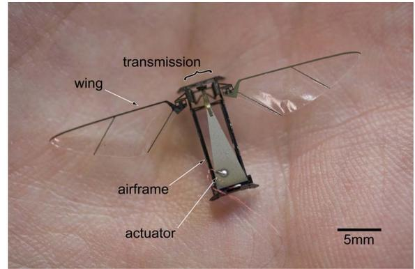
Fig. 24. Photograph of the flapping-wing flying microrobot used in the hovering experiments.
