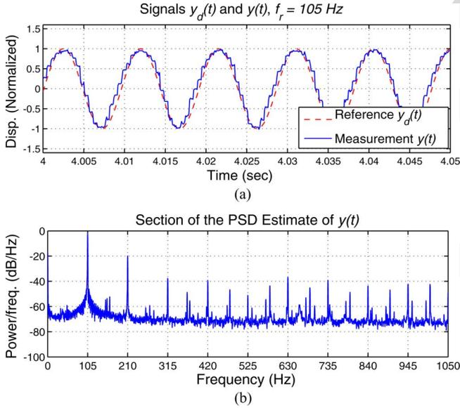
Fig. 10. Case 4. *Upper Plot*: Time series of  $y_d(t) = A_r \sin(2\pi f_r t)$  and  $y(t)$ , using the model-based adaptive scheme in Fig. 6, with  $A_r = 1$  and  $f_r = 105$  Hz. *Bottom Plot*: PSD estimate of the measured output  $y(t)$ .
