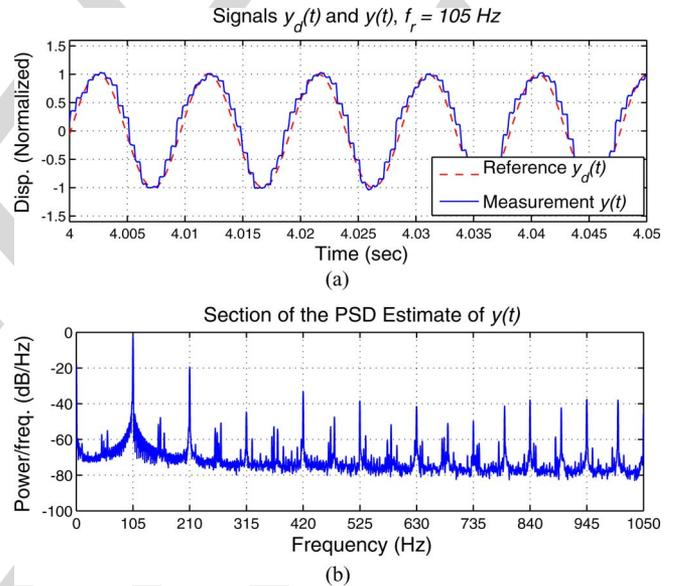
Fig. 8. Case 2. *Upper Plot*: Time series of  $y_d(t) = A_r \sin(2\pi f_r t)$  and  $y(t)$ , using the adaptive scheme in Fig. 5, with  $A_r = 1$  and  $f_r = 105$  Hz. *Bottom Plot*: PSD estimate of the measured output  $y(t)$ .
