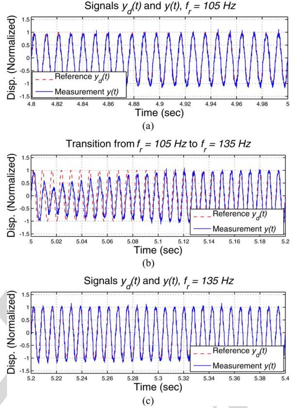
Fig. 19. Experimental example of a time-varying reference frequency  $f_r$ . This case shows in red the transition of  $y_d(t) = A_r \sin(2\pi f_r t)$  from  $f_r = 105$  Hz to  $f_r = 135$  Hz at  $Time = 5$  s. The resulting measurement  $y(t)$  is shown in blue.
