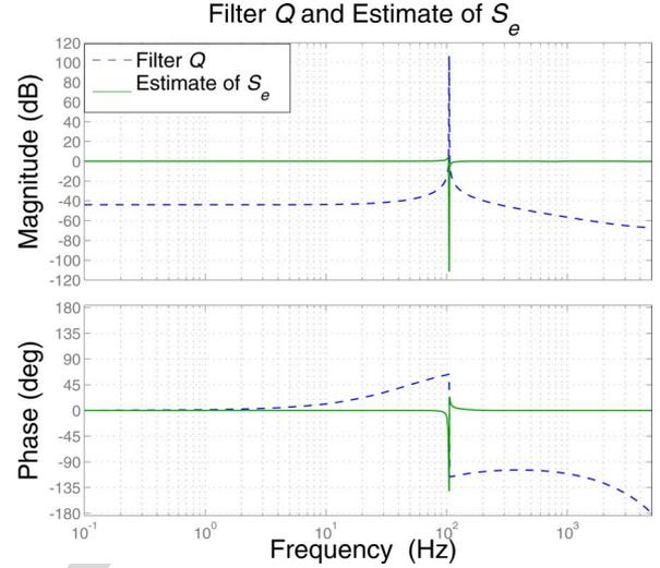
Fig. 12. Filter  $Q(z)$  and estimate  $\hat{S}_e(z) = [1 - \hat{P}(z)Q(z)]^{-1}$  of the error sensitivity function  $S_e(z)$ , using the LTI equivalent representation associated with Case 2.
