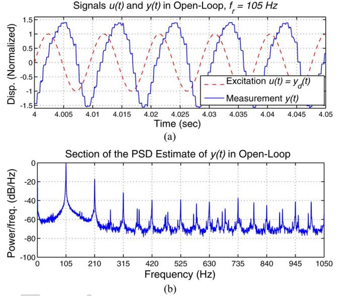
Fig. 7. Case 1. *Upper Plot*: Time series of  $u(t) = A_r \sin(2\pi f_r t)$  and  $y(t)$  in open loop, with  $A_r = 1$  and  $f_r = 105$  Hz. *Bottom Plot*: PSD estimate of the measured output  $y(t)$  in open loop.
