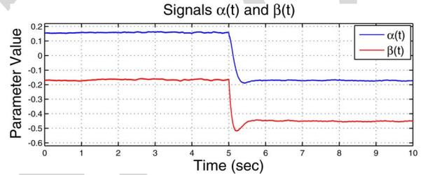
Fig. 20. Evolution of the adaptive parameters  $\alpha(t)$  and  $\beta(t)$ , corresponding to the experiment in Fig. 19. The first 5 s show the parameters in steady state, with  $f_r = 105$  Hz. At  $Time = 5$  s the value of the reference frequency  $f_r$  is changed from 105 Hz to 135 Hz. From  $Time = 5$  s to  $Time = 10$  s the plot shows the parameters' transition until they reach steady state, with  $f_r = 135$  Hz.
