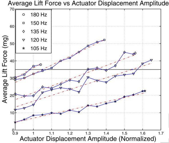
Fig. 17. Empirical relationship between the average lift force and the actuator displacement amplitude, with  $f_r$  taking the values 105, 120, 135, 150, and 180 Hz.
