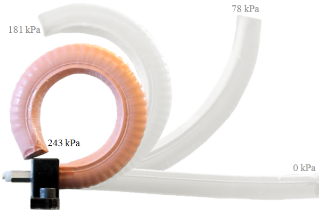
Fig. 4. Range of motion of the fiber reinforced soft bending actuator constructed from 28A durometer rubber (see Table I for material properties).
