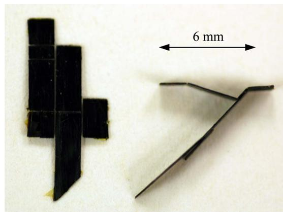
Fig. 7 Flat and Fully Assembled Slider Crank Leg
