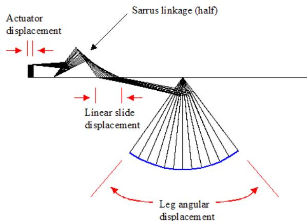
Fig. 2 Motion of the Leg Driving Mechanism
