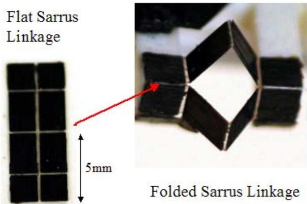
Fig. 6 Flat and Fully Assembled Sarrus Linkage
