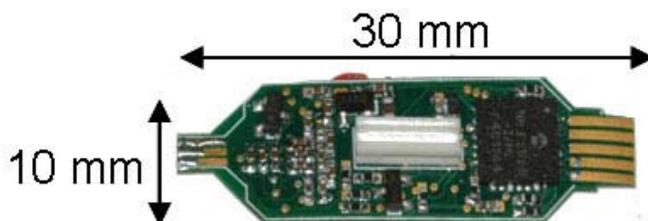
Fig. 10 Lightweight power and control electronics board
