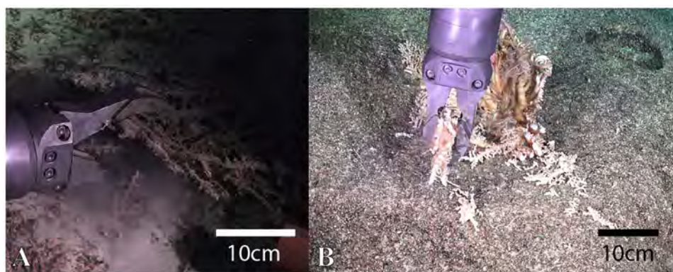
Fig 11. Challenges when grasping brittle specimens with hard bodied manipulators. A: Coral rubble (depth: 616m, S1 Video). B: Enallopsammia sp. coral (depth: 434m).
