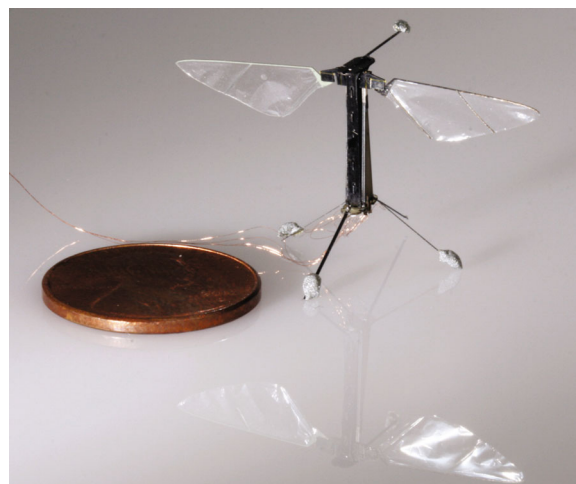
Fig. 1 Photograph of one of the flapping-wing flying micro-robots used in the work presented in this paper. The prototypes considered in this work have two completely independent actuators used simultaneously for power and control. The ball-shaped markers glued to the robot are used by a Vicon motion capture system in the estimation of position and orientation of the robot. This robotic prototype was entirely developed and fabricated at the Harvard Microrobotics Laboratory
